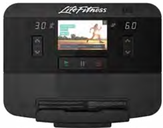
INTEGRITY X CONSOLE The X Console offers a 7" touch screen and engaging workout experience through NFC and Bluetooth® connectivity.
