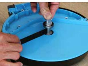
**6** *Take the new strap and guide it through the small opening in the axis. Make sure the strap is inserted far enough and place the pen back into the loop.*
