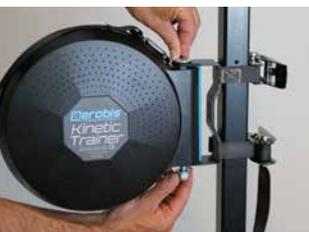
**7** *Pull the strap tightly so the pen is fixed in the axis. The Kinetic Trainer can be assembled again.*
