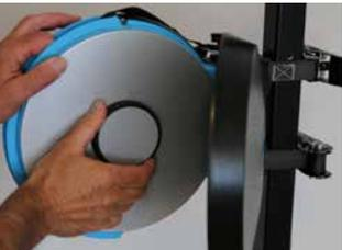
**6** *Proceed in reversed order. Place the new disc on the axis, and fasten the quick release knob. At your discretion, first fasten knob and then close the door or the other way around.*
