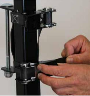
**4** *The strap can now be tightened by moving the ratchet back and forth. On average, make 1.5 to 3 strokes.*
