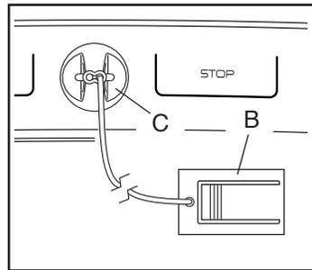
**key can be pulled from the console, causing the walking belt to slow to a stop. Test the clip by taking a few steps backward; if the key is not pulled from the console, adjust the position of the clip.**
