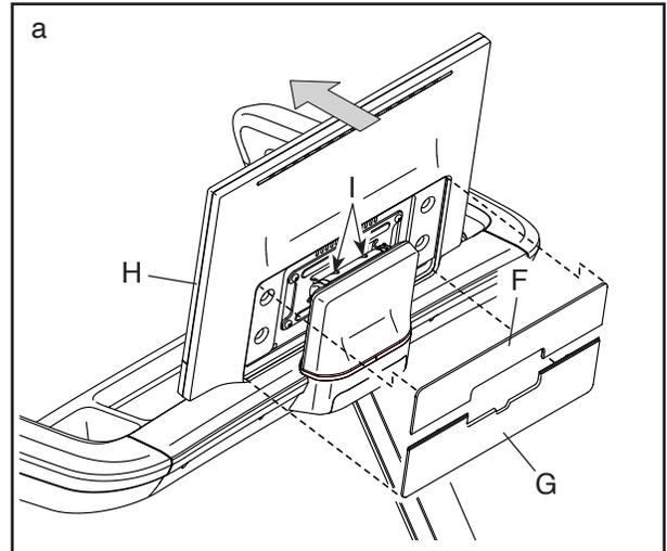
Next, tilt the top of the console (H) in the direction shown by the arrow, and use one of the included hex keys to tighten the two indicated M6 x 15mm screws (I) a small amount.
