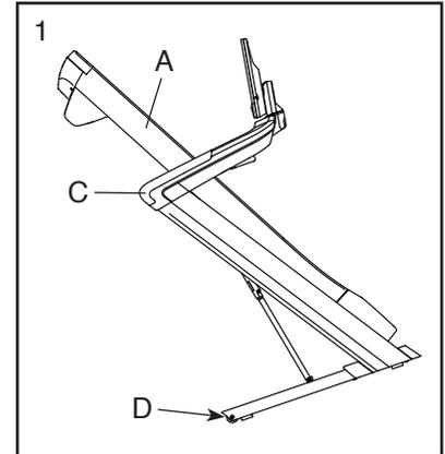
2. Pull back on the handrail (C) until the treadmill will roll on the wheels (D), and carefully move it to the desired location. **CAUTION: Do not move the treadmill without tipping it back, do not pull on the frame, and do not move the treadmill over an uneven surface.**
