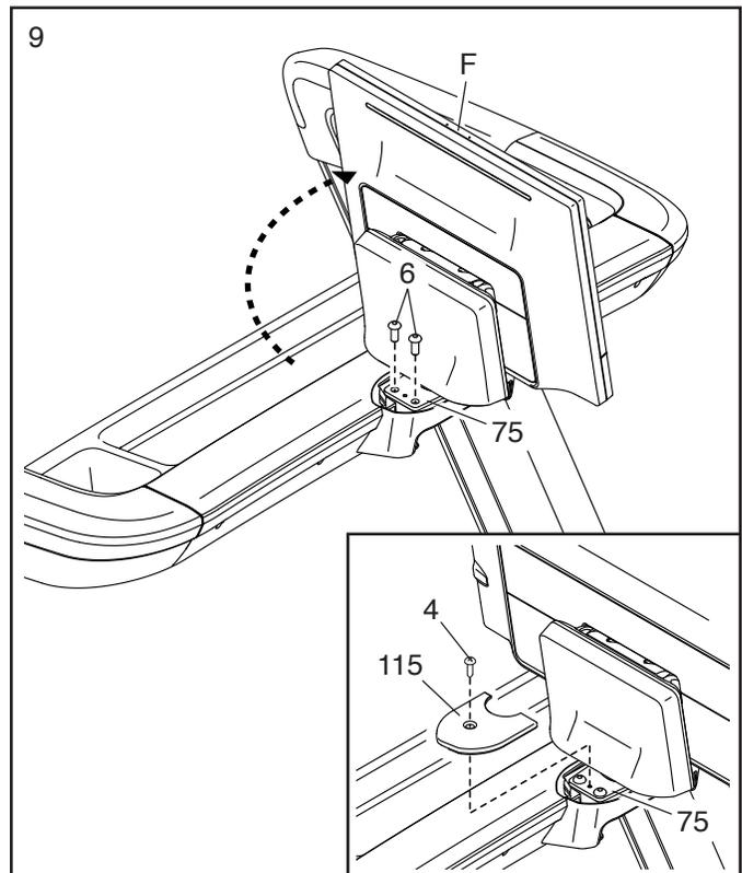
10. **Rotate the console assembly (F) back to its original position.** Firmly tighten the two 5/16" x 3/4" Screws (6) that you attached in step 8.
