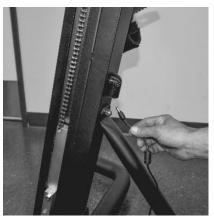
**20.** Plug the transformer into the back of the post and a 110 volt wall socket.
