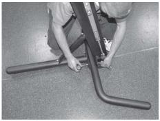
**10.** Attach back tubular floor brace to post with (2) hex head bolts  $3/8'' \times 3\frac{3}{4}''$  long and (2) lock nuts. **DO NOT TIGHTEN FULLY AT THIS TIME.**
