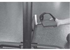
**15.** Attach foot pedals with "L" shape bracket pointing up, using (2) 3/8" x  $1 \frac{1}{2}$ " long hex head bolts.
