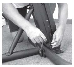
**12.** After tubular brace is in place, go back and **FULLY TIGHTEN** the (2) 3 <sup>3</sup>/<sub>4</sub> long base bolts.
