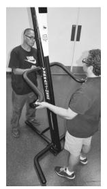
**17.** Attach side handrails with (3) hex head bolts 4" long and (3) 3/8" lock nuts.
