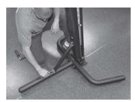
**14.** Next, tighten the **<u>BOTTOM</u>** lock nut on the back brace to complete post assembly.
