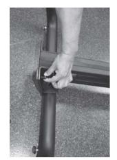
**7.** Screw in (4) self tightening base bolts.
